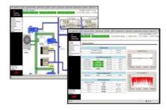
The Air System Controller (ASC) is a system automation product developed specifically for complex compressed air systems and the integration of virtually all equipment and instrumentation found in air systems throughout a broad range of industry. The primary goal of the ASC is to provide data acquisition and display for health monitoring and energy management for control and air system optimization.
