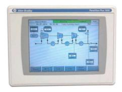
Custom PLC-based systems are used for packages with high input/output (I/O) counts, multiple gas circuit control loops, and multiple processes. PLC solutions available from most major industrial suppliers. Our engineers can design, program and supply your specified PLC system mounted and wired to any compressor package.
